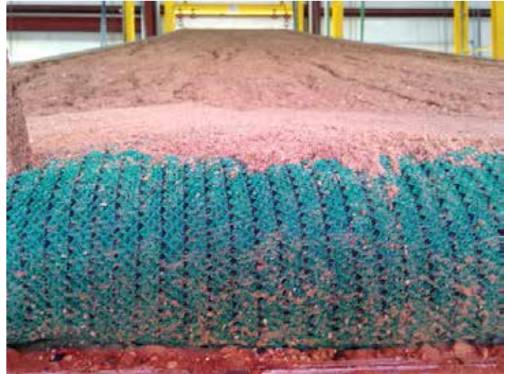
Figure 1: Testing of 5-inch SiltSoxx
