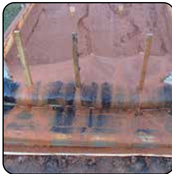
Fig. 3: 12" Off-Spec Compost Sock (66% Removal Efficiency)
