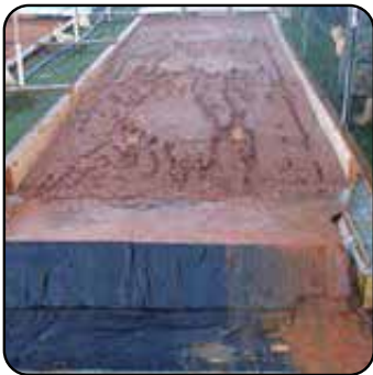
Fig. 5: 10" Triangular Silt Dike (93% Removal Efficiency)
